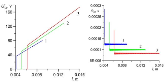
Fig. 4. Diagrams of changes of parameters of arc having the stretched plasma column and described using the Cassie-Voronin model:  $(1 - (p_v = 40 \times 10^6 \text{ Wm}^{-3}, l = (4 + 5t) \times 10^{-3}, \text{m}), 2 - (p_v = 50 \times 10^6 \text{ Wm}^{-3}, l = (5 + 8t) \times 10^{-3}, \text{m}), 3 - (p_v = 60 \times 10^6 \text{ Wm}^{-3}, l = (6 + 10t) \times 10^{-3}, \text{m}))$ : a) voltage  $U_{cl}$  and b) damping function  $\theta_{cl}$
