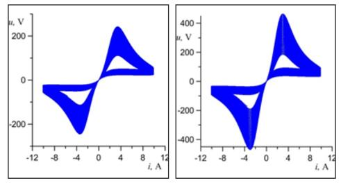
Fig. 1. Dynamic current-voltage characteristic of arc having the stretched plasma column and described using the Mayr-Voronin model: a) parameters  $(p_v = 6 \times 10^8 \text{ W/m}^3, l = (4 + 5t) \times 10^{-3}, \text{ m})$  and b) parameters  $(p_v = 7 \times 10^8 \text{ W/m}^3, l = (5 + 8t) \times 10^{-3}, \text{ m})$
