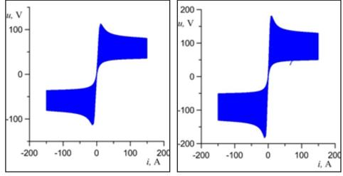
Fig. 3. Dynamic current-voltage characteristic of arc having the stretched plasma column and described using the Cassie-Voronin model a) parameters ( $p_v=40\times10^6$  Wm<sup>-3</sup>,  $l = (4 + 5t)\times10^{-3}$ , m) and b) parameters
