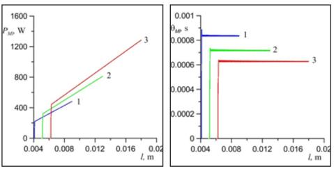
Fig. 2. Diagrams of changes of parameters of arc having the stretched plasma column and described using the Mayr-Voronin model:  $(1 - (p_v = 6 \times 10^8 \text{ W/m}^3, l = (4 + 5t) \times 10^{-3}, \text{ m}), 2 - (p_v = 7 \times 10^8 \text{ W/m}^3, l = (5 + 8t) \times 10^{-3}, \text{ m}), 3 - (p_v = 8 \times 10^8 \text{ W/m}^3, l = (6 + 12t) \times 10^{-3}, \text{ m})):$ a) power  $P_{Ml}$  and b) damping function  $\theta_{Ml}$
